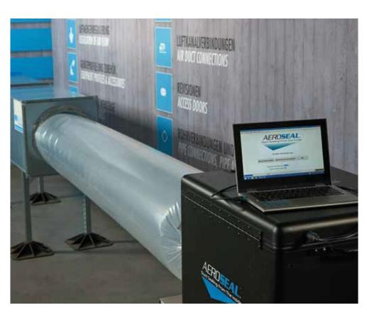
The process itself needs only a few steps of preparation. First all inlets and outlets of the air duct system are sealed shut with foam plugs or metal plates. The ductwork connections to air handling units, fans or heat exchangers are dis-connected and built-in sensors are taped over, so that no particles of the sealant can get into these
