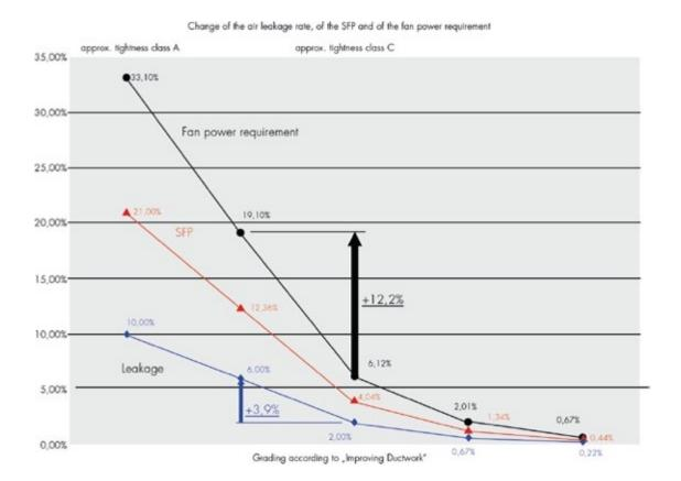
Fan power requirement increases by 3 times compared to the air leakage rate.
